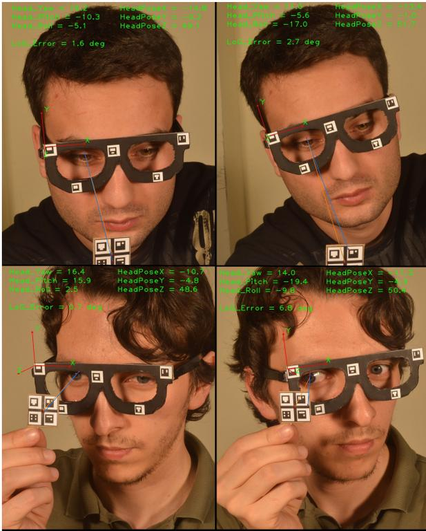
Figure 4. Sample results with position, orientation and error numbers from low and high error examples. The blue line is the estimated LoG, the orange line is the ground truth.
