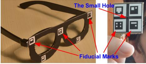
Figure 2. left: the modified 3D movie glasses, right: the target with the small hole.
